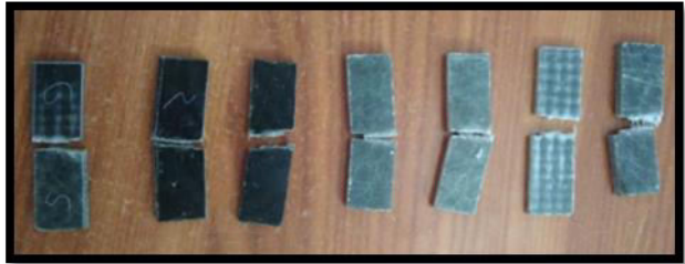
Figure 42 impact strength specimens of all materials
