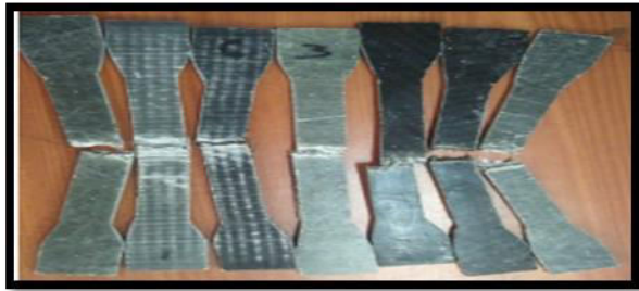
Figure 40 tensile strength materials specimens The percentage of elongation is calculated by the follow equation
