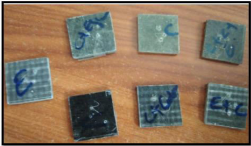
Figure 43 hardness testing specimens
